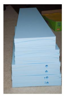
The foam material for the individual aircraft components may come out of the box like this photo to the left, in which case the builder would have to cut and shape the foam into the correct finished contour and form. Most composite kits provide the type of foam cores as shown below, with the foam cores properly shaped and sized, ready for application of fiberglass cloth and resin.
