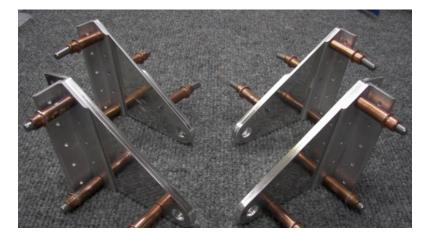
Aileron Brackets after trimming and drilling
