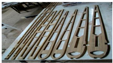
This photo shows horizontal stabilzer parts as provided by the factory. As such the builder will receive minor credit for fabrication.
