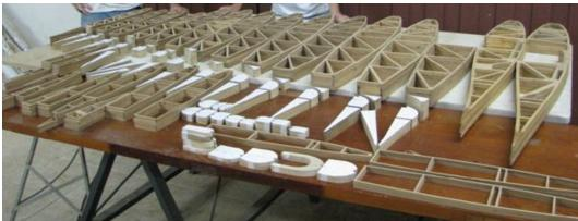
Wood Kit Wing and Empennage Components prefabricated at factory.
