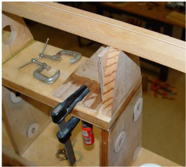
Spar and leading edge rib joining
