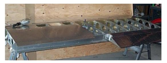
In the photo above, the aileron (fabricated and assembled at the factory) has been attached to the left wing (wing is upside down) by the builder.
