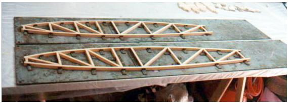
Ailerons constructed from plans and raw materials using a template/jig
