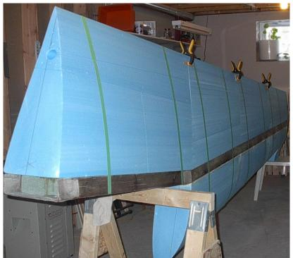
Wing Foam Core mated to carbon fiber spar
