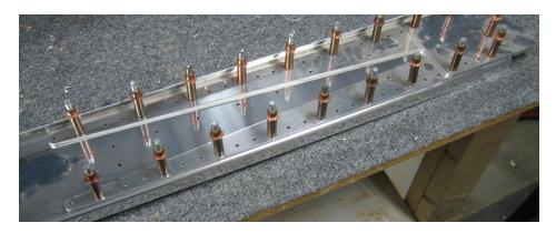
Wing Rear Spar with reinforcement plate in place with clecos
