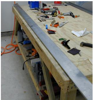
Task W1 covers both the main and rear spars and in this case, the rear spar requires a significant amount of work on the builder's part. First there is the trimming, deburring and holes to drill. Then reinforcement plates and brackets must be attached.
