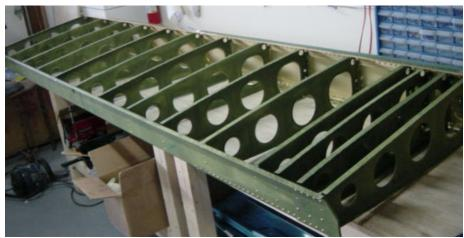
Basic or Primary Wing Structure; main and rear spars joined to middle/main ribs with zinc chromate primer.
