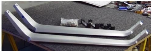
Aluminum Landing Gear Struts from the factory
