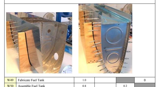
In this kit (quickbuild), the fuel tanks are integral to and come built into the wing leading edge at the factory (optional) and although separate and distinct fuel tank does not exist, since the extra steps, sheet metal and sealant applied create a resevoir it can be scored. In the quick build kit, this is all done at the factory. The builder received minor assembly credit in W50, for bracket attachment and some other minor applications.
