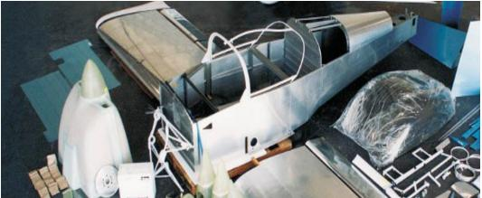
Quick build Kit with Quick build Fuselage
