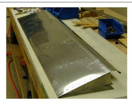
The flap on this aircraft does not have a conventional leading/trailing edge. The design extends the top flap skin past the spar in the front to cover the gap between the flap and wing. At trailing edge, the rear of the top skin folds down and under to overlap and then attach to the bottom skin.
