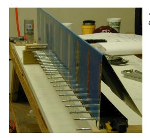
Aileron skin being joined to the aileron spar in task W25.
