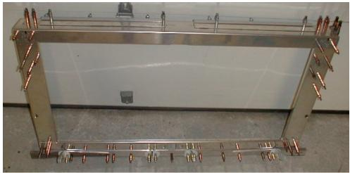
Fuselage Forward Bulkhead to which the firewall will attach.
