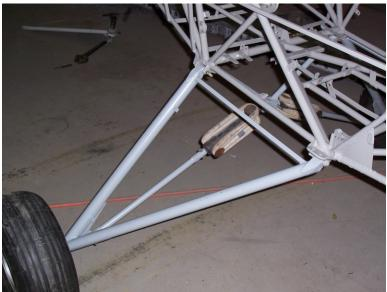
Steel Tube and bungy system used on Cub-like aircraft kits
