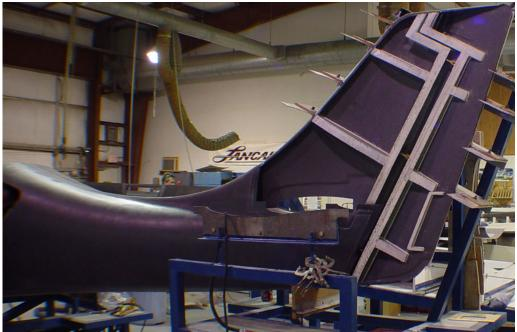
Rear Fuselage with integrated Vertical Stabilizer and attached Rudder
