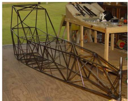
Steel Tube Fuselage prefabricated at the factory.
