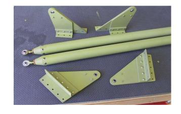
Aileron Brackets and Fittings are largely fabricated at the factory but need to be trimmed, drilled, deburred and riveted (assembled) in place. The aileron bell crank is provided but will be installed (assembled to) in the wing by the builder
