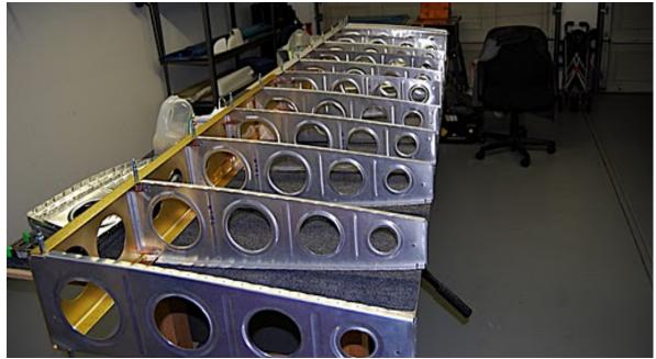
Main Spar with middle ribs attached.
