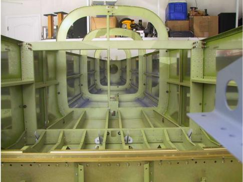
Standard Kit Fuselage structure assembled
