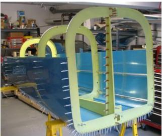
panels to the fuselage structural components. This photo shows that the fuselage basic structure construction progresses in conjunction with the assembly of the skin in true semi-monocoque fabrication.
