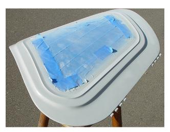
There are two fuselage window just behind the cockpit. Both are framed and fit to plexiglass. At least one has a hinge and latch mechanism for opening into the baggage area. The frames are cut and shaped by the manufacturer but require trimming, sanding, and bonding on both windows by the builder to complete the fabrication process. The scores may appear as such below.
