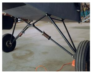
Spring and Steel Landing Gear
