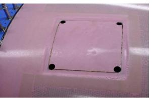
Composite cowling with hinge clecoed in place
