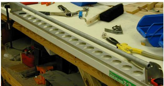
Aileron Spar with Counterbalance bar and end brackets
