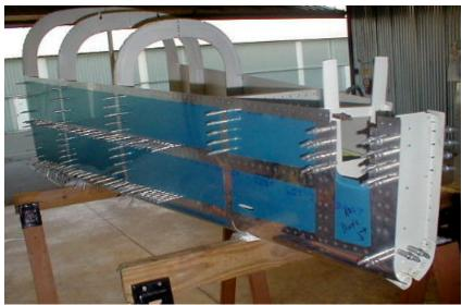
Aft Fuselage Section Standard Build Kit
