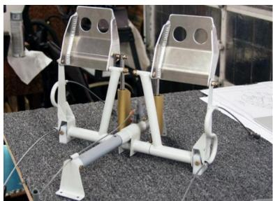
Rudder Pedals and Pivot Tubes
