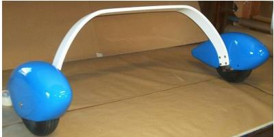
Composite (Carbon Fiber) Spring Landing Gear
