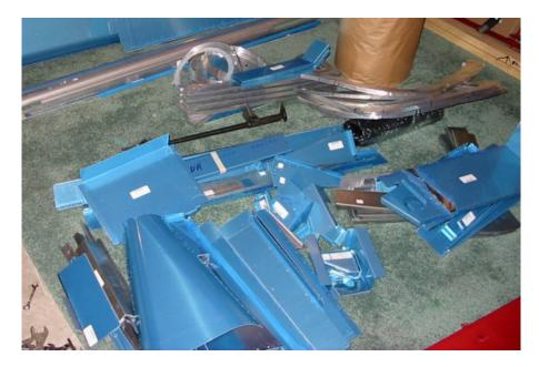
The sheet metal skin panels provided in the kit for the fuselage are cut to the exact size and predrilled for their individual attach points. The builder still has to trim, debur and up drill and probably dimple the skin to prep for assembly to the basic fuselage structure. There will also be some reinforcement braces and stiffeners to drill and attach.
