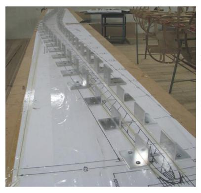
This photograph shows a template for a wing spar. This is substantial evidence that the spar is made from raw materials (i.e., wood in this case) since there would be no need to provide plans for a template/jig if the wing spar was provided with the kit either partially or wholly completed.
