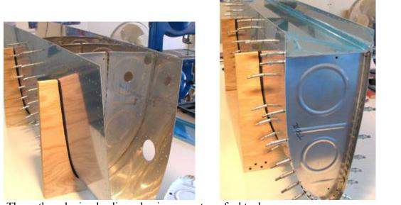
The outboard wing leading edge incorporates a fuel tank.
