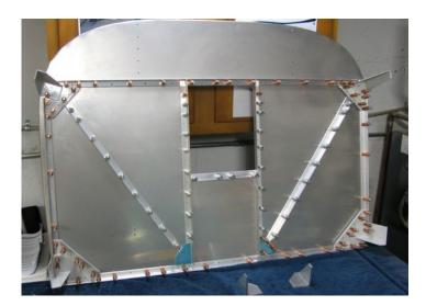
The firewall with angles, stiffeners, brackets and gussets clecoed in place for final riveting. The builder was required to cut and drill some of the braces and angles and then had to cut the square hole in the center. Finally he had to rivet all the parts together to make the finished firewall component seen in the photo to the left.
