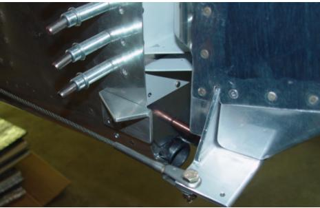
Rudder Cable attached to Rudder Horn
