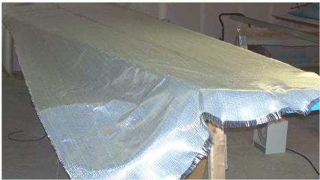
Fiberglass cloth laid out for cutting and layup
