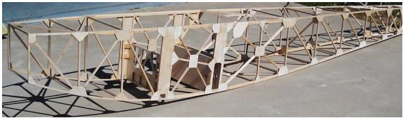
Basic wood fuselage internal structure
