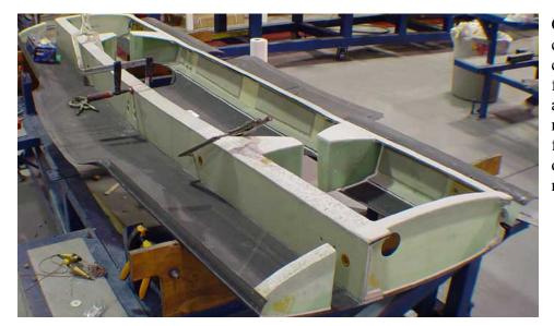
Center wing section, composite construction, fabricated in a mold at the factory. All materials, spar, ribs, formers are all made out of composite material.
