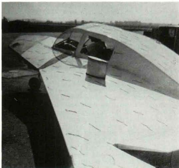
Airflow tests on the "Delta" were made with tufts attached over the airplane, and the flow can be observed here with the engine running. Note an earlier style windshield and canopy arrangement installed at this time.
